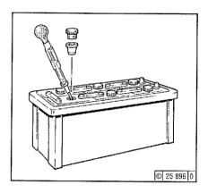
Measure electrolyte density of individual cells with commercial hydrometer.
