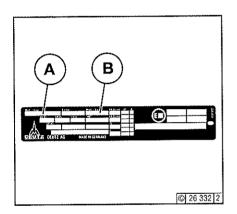
The model  ${\bf A}$ , the engine serial number  ${\bf B}$  and the performance data are stamped on the rating plate.
