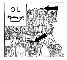
As a rule, engines are delivered without oil. Pour lube oil into the oil filler neck (arrow). For oil grade and viscosity, see 4.1.
