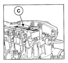
The rating plate  ${\bf C}$  is attached to the valve cover.
