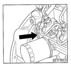
The engine serial number  ${\bf B}$  is stamped on the crankcase  ${\bf D}$  as well as the rating plate.
