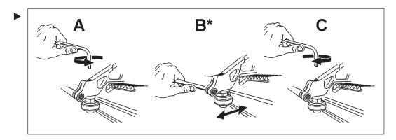
\* The guide rollers are set correctly when they align in the guide groove and it is possible to turn them by hand.
